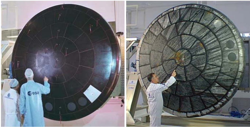
Figure 8: ARD Front-Shield TPS before and after recovery.
